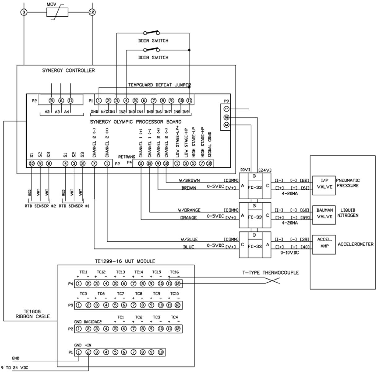
**Figure 5 Typical Retransmit Converter Application Drawing**
