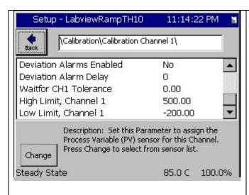
Other Parameters in the Channel Calibration Screen.
