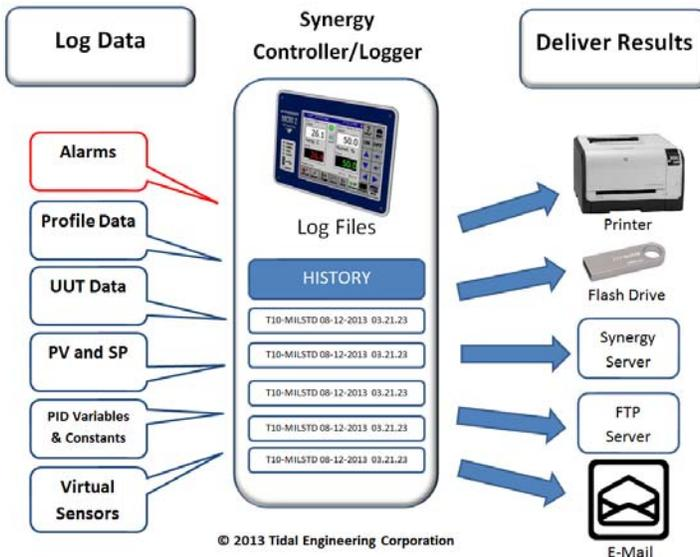
The logging system captures alarms and chamber control performance data as well as UUT Thermocouple data:
