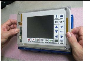
Remove the (5) screws securing the touch screen support and unplug the flex cable for the touch sensor as shown below.
