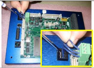
Remove the (10) screws and lift the LCD panel out of the case.
