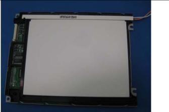
Lift the lamp housing and remove it from the display and pull the white lead from the lamp housing as shown below.
