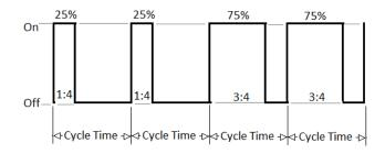
In addition to staging, the PWM Time-Proportioning Outputs can be used to control any system or user functions requiring a general-purpose Time proportioning control signal. Setpoints, process data, constants, and internal PID values can be transmitted this way. The PWM Retransmit Feature provides programmable scaling and can be controlled thru a set of communication commands or APIs.
