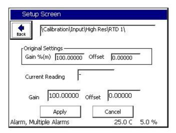
Alternatively, for End-to-End temperature Calibration, a reference temperature reading is compared against the Synergy Controller reading. This takes into account and corrects for the sensor and controller characteristics.
