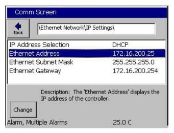
Connect all the Synergy Controllers with Ethernet cables and assign the TCPIP addresses either statically (preferred) or using DHCP. See the Synergy Controller IP Settings screen below:
