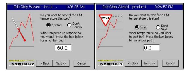
The tolerance for each channel is specified on a channel-by-channel basis in the Setup Screen shown below. The Wait-For step doesn't control the setpoints during the step. The setpoints during the WaitFor step are determined by the setpoints of the prior step and are held constant for the duration of the step.
