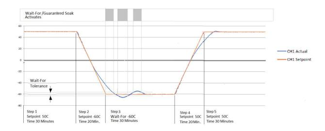
Note that the setpoints during the WaitFor step are determined by the final setpoints of the prior step and are held constant for the duration of the step. This is true both if the WF Guaranteed Soak Mode is enabled and if it is disabled.
