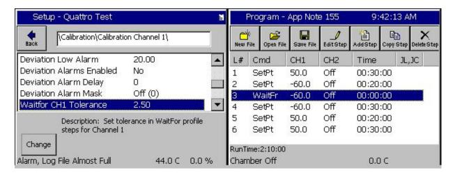
In the figure below, Step 3 is the Waitfor Step. The program waits at Step 3 until the temperature is in Tolerance.
