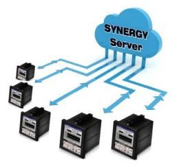
The Synergy Server is a web server application designed to provide virtually unlimited centralized and searchable storage for an unlimited number of Synergy Controllers. Based on Virtual open source LAMP server technology (Linux OS, Apache Web Server, MySQL Database, and PHP scripting platform), the Synergy Server provides centralized storage and a simple Web Interface for:
