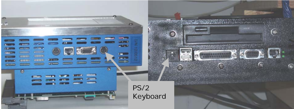
PS/2 Keyboard Connector on a Synergy Controller (left) and VersaTenn V (right)
