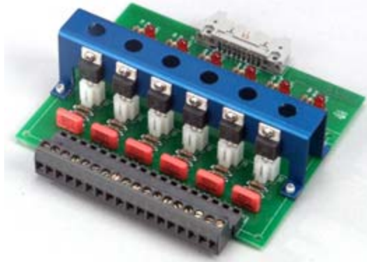
TE1151-6 Triac Output Board Schematic
