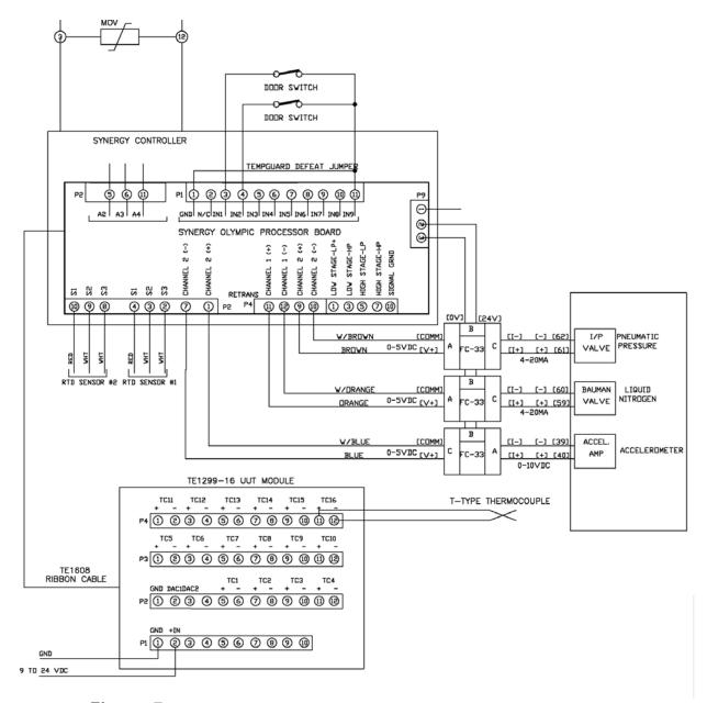
Figure 5 Typical Retransmit Converter Application Drawing
