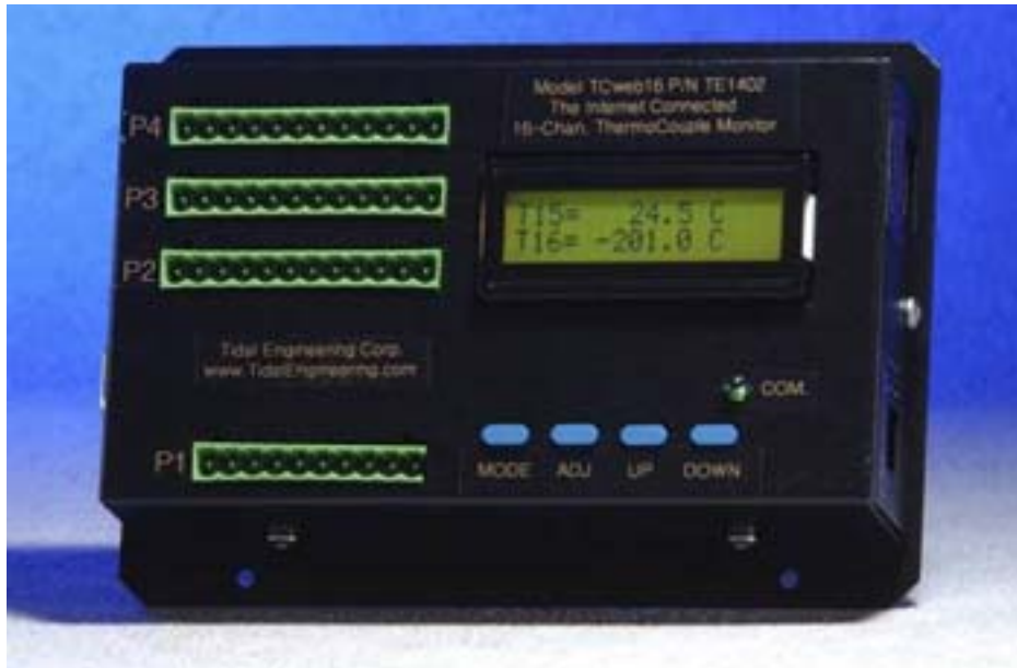
Figure 1 TCweb Thermocouple Monitor
